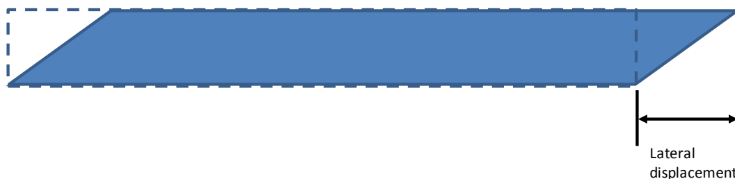
Figure 2. Simple shear test piece. Strain is applied via the lateral displacement of the grips, resulting in skewing of lines originally perpendicular to the lateral displacement.
