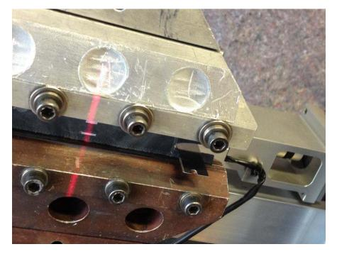
Carefully controlled cutting of a pre-strained elastomer specimen with an instrumented blade provides an effective way to observe the material's endurance limit.
