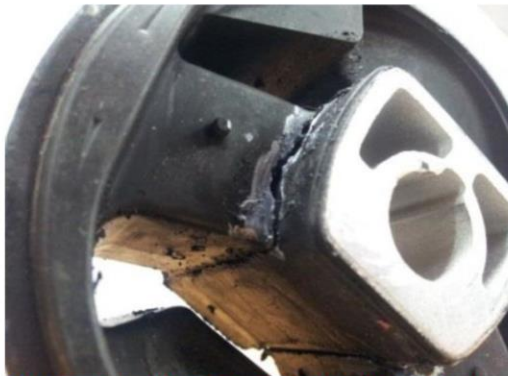
Observed bushing failure mode (front view)
