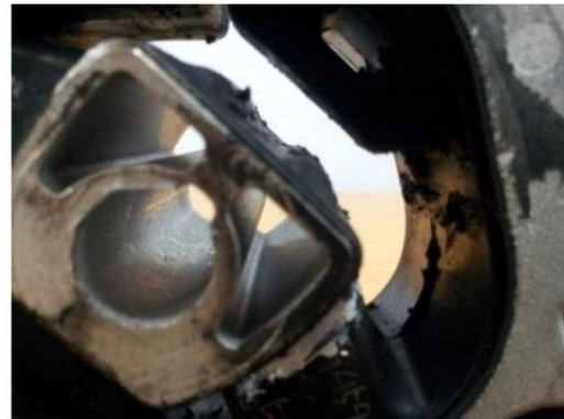
Observed bushing failure mode (rear view)
