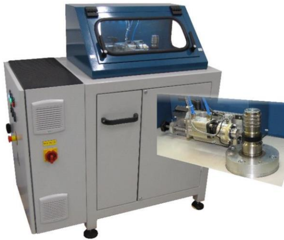
LEFT: Photograph of Instrumented Chip & Cut Analyser (ICCA), showing expanded view of impacting device and sample. RIGHT: Plot of chip & cut propensity ( P ) versus number of impact cycles for NR/BR(75/25) compounds reinforced with 50 phr and 65 phr of N339 carbon black.
