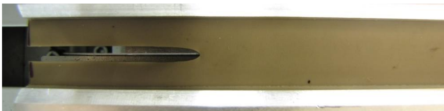
Figure 5. Blade-loaded, edge-cracked planar tension specimen under load during cutting on the Coesfeld Intrinsic Strength Analyser.
