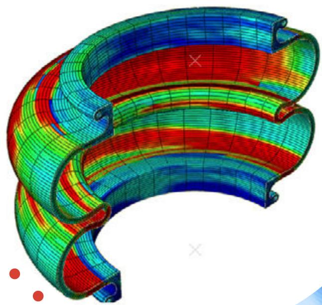
Give Endurica CL<sup>TM</sup> a finite element simulation of your loading history, specify your material(s), then CL computes the fatigue life of your rubber part.
