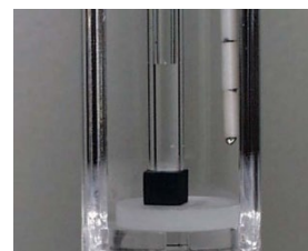
Thermal expansion is measured using thermomechanical analysis (TMA).
