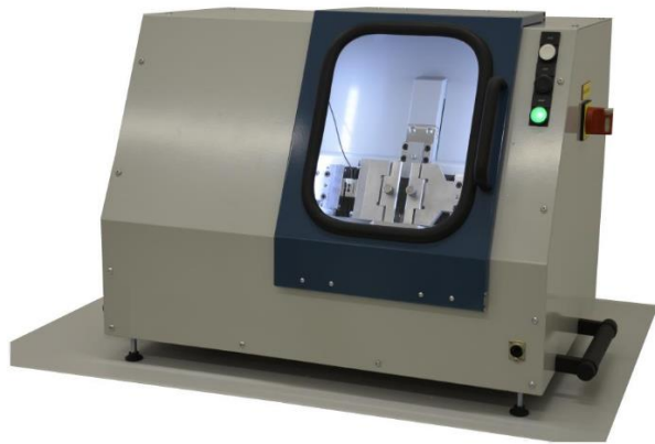
LEFT: Picture of the Coesfeld Intrinsic Strength Analyser. RIGHT: Method used to determine intrinsic cutting energy ( S_{0,c} ) from cutting energy versus tearing energy data.
