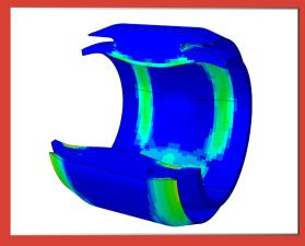
Durability simulations are a key component of the engineering package Tenneco uses to win new business from their OEM clients. The ability to efficiently and accurately simulate road loads, block cycle schedules, and multiaxial, variable amplitude load inputs as part of routine production engineering workflows sets Tenneco apart from its competition.
