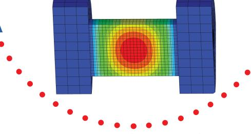
Endurica MP helps identify and avoid the "blowout" failure mode. "Blowout" or thermal runaway is caused by self-heating arising from viscoelastic and thermochemical mechanisms. The graph below shows the transient history of temperature rise in a rotating beam bending test specimen used by the Coesfeld Heat Build Up Analyser. The exothermic release of heat energy during the test leads to a reversion / blowout failure that can be simulated with Endurica MP.
