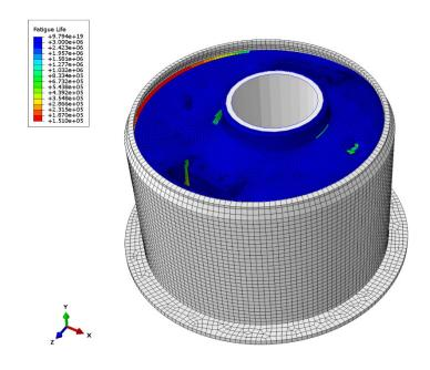
The hex-dominated mesh produced by Coreform Cubit's meshing software facilitates accurate life predictions with Endurica.
