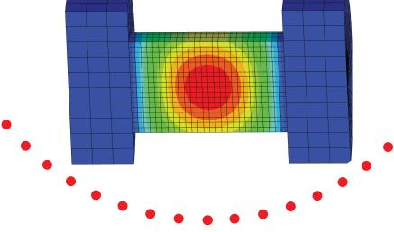
Endurica MP helps identify and avoid the "blowout" failure mode. "Blowout" or thermal runaway is caused by self-heating arising from viscoelastic and thermochemical mechanisms. The graph below shows the transient history of temperature rise in a rotating beam bending test specimen used by the Coesfeld Heat Build Up Analyser. The exothermic release of heat energy during the test leads to a reversion / blowout failure that can be simulated with Endurica MP.
