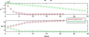
The evolution of tear strength T<sub>c</sub> and stiffness E with ageing depends on oxygen availability.
